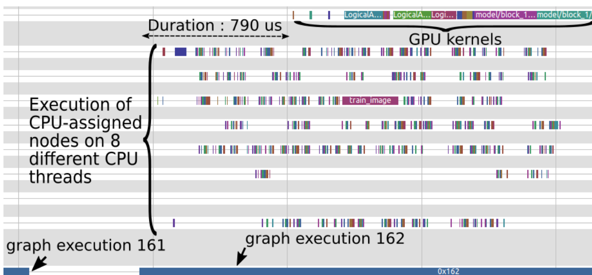
Figure 4.8 Execution with the two optimizations : setting num_parallel_calls to 8 and prefetch to 1. In addition to the parallelization of CPU work, pipelining has been added and increases again the performance.
