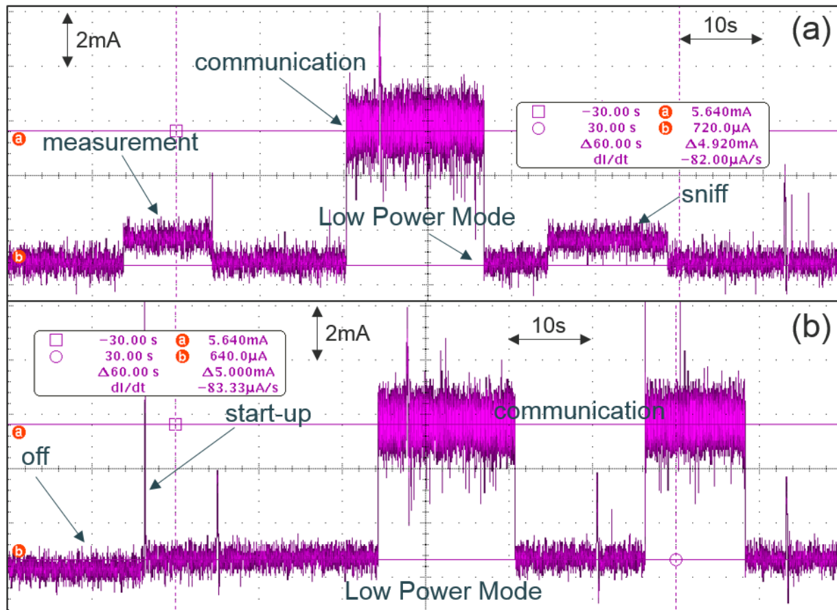
Figure 3-8 Current consumption in the different operating modes (a) and in a regular example use (a) of the communication implant.
