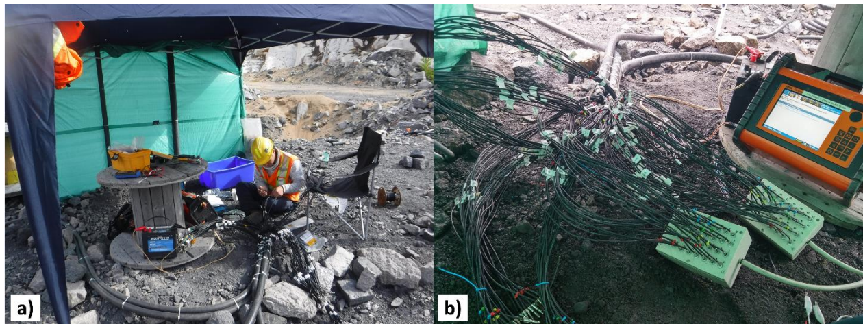
Figure 4-2: Geophysical equipment set-up in the field. a) Location where ERT monitoring is performed. b) 64 cables connected to the connection boxes and ABEM Terrameter LS .
