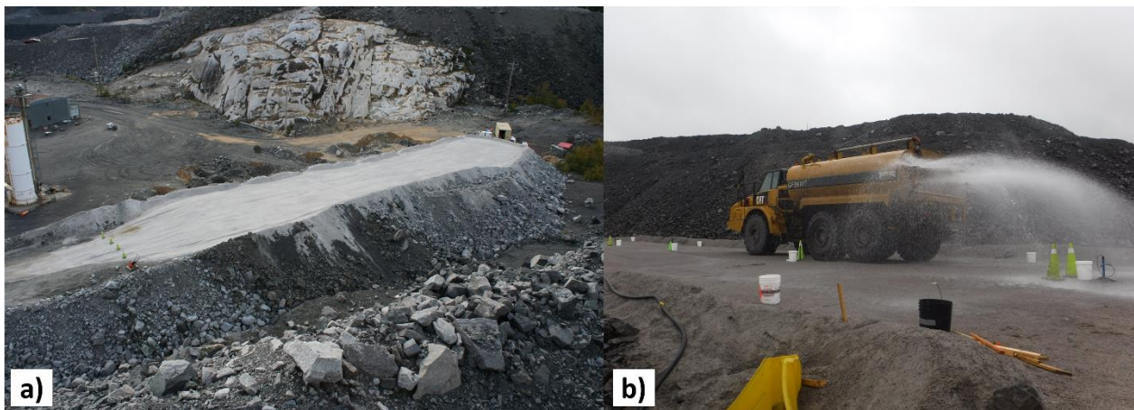
Figure 4-3: a) Global view of the experimental waste rock pile, and b) infiltration test using a water truck.
