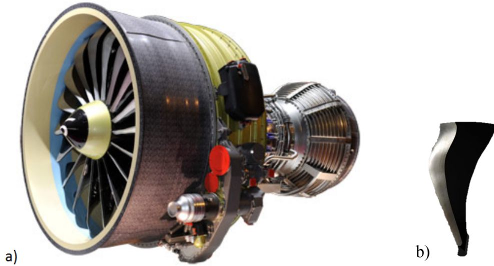
Figure 1.1 a) LEAP engine of Safran group (Julian, 2013-11-16) - b) Single fan blade made of 3D woven composites used in the LEAP engine (Drouin, 2017)
