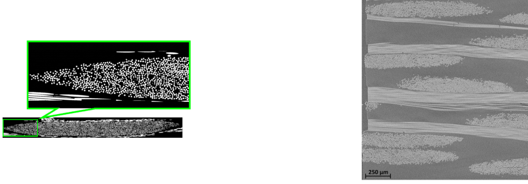
Figure 2.13 a) Microscopic transversal cross-section of a yarn (Lapeyronnie et al. , 2011)- b) Tomographic scan of a composite material (Madra et al. , 2017)
