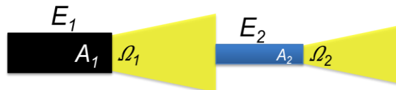
Figure 3-16: The etendue is determined by the emission area of a source and the solid angle of the light cone. For example, 100% of the light would pass from one section of the system to the next one if the ratio of their etendues ( E_2/E_1 ) was 1.
