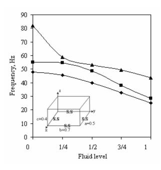
Fig. 11: Variation of frequencies of a perimetrically simply supported bottom reservoir versus fluid level variation
