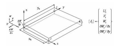
Fig. 1: Flat rectangular shell element
