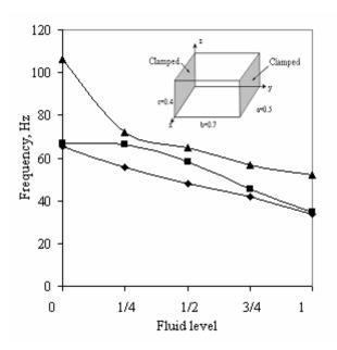
Fig. 7: Variation of frequencies of reservoir with two parallel clamped walls versus fluid level variations
