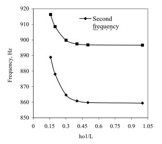
Fig 14-b: Variation of  $2^{nd}$  and  $3^{rd}$  frequencies as a function of  $h_{o1}$  variations at sufficiently large  $h_{o2}$
