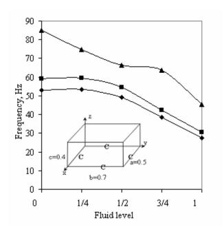
Fig. 9: Variation of frequencies of a perimetrically bottom clamped rectangular reservoir versus fluid level variations
