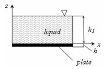
Fig. 3: Fluid solid element having free surface at  $z=h_I$
