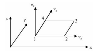
Fig. 2: Coordinate transformation for rectangular element
