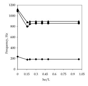
Fig 16: Variation of frequency as a function of simultaneous changes in  $h_o$ , where  $h_o = h_{o1} = h_{o2}$
