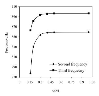
Fig 15-b: Variation of  $2^{nd}$  and  $3^{rd}$  frequencies as a function of  $h_{o2}$  variations at sufficiently large  $h_{o1}$
