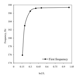
Fig 15-a: Variation of  $1^{st}$  frequency as a function of  $h_{o2}$  variations at sufficiently large  $h_{o1}$
