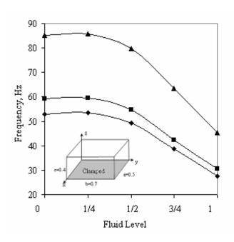
Fig. 6: Variation of frequencies of bottom-clamped reservoir versus fluid level variations
