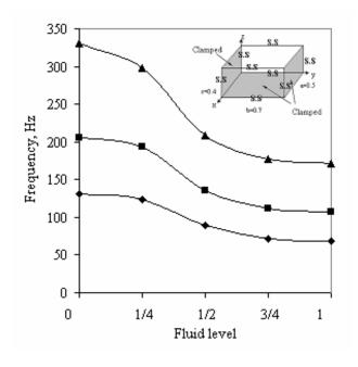
Fig. 10: Variation of frequencies of a reservoir with two facing walls and bottom clamped and two other walls simply supported at edges versus fluid level variations
