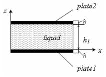
Fig. 4: Two identical plates coupled with bounded fluid
