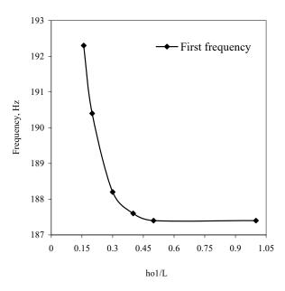
Fig 14-a: Variation of  $1^{\text{st}}$  frequency as a function of  $h_{\text{o}1}$  variations at sufficiently large  $h_{\text{o}2}$
