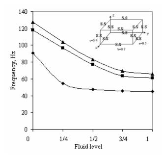
Fig. 12: Variation of frequencies of a simply supported reservoir at all edges versus fluid level variations
