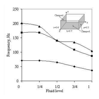
Fig. 8: Variation of frequencies of reservoir with two facing walls and bottom clamped versus fluid level variations
