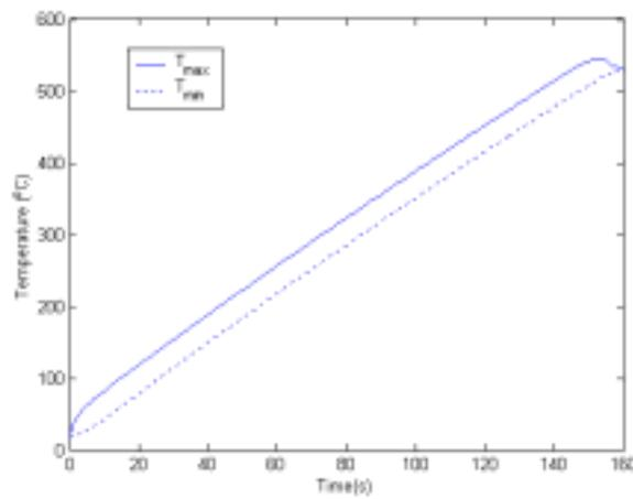
FIG.11.3: Evolution of Surface and Central Temperature
