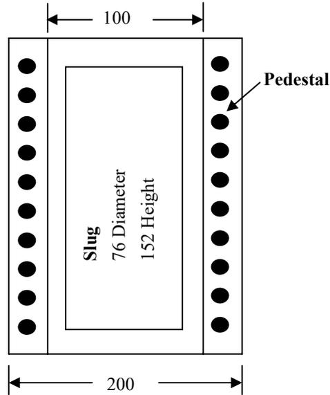
FIG. 1 Schematic of Induction Heating Coil and Slug
