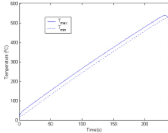
FIG.12.3: Evolution of Surface and Central Temperature
