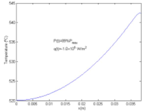
FIG.5.2: Surface-to-Core Profile
