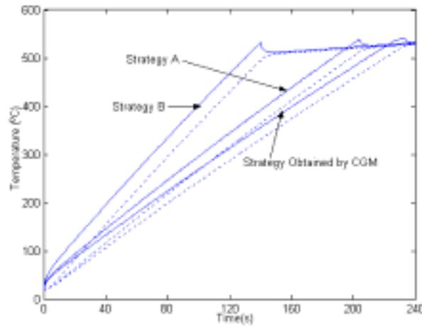
FIG.9.3: Evolution of Surface and Central Temperature
