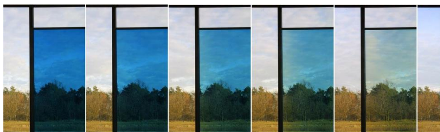
Figure 1.3: Coloration sequence of an electrochromic window [57].
