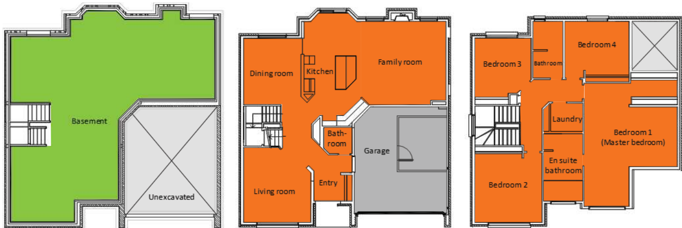
Figure 4 Heating zones for mechanical thermostat
