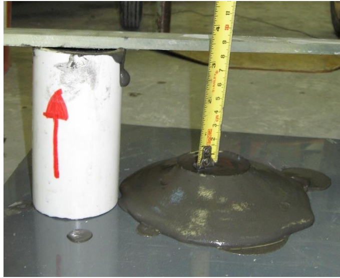
Figure 3.4: Example of slump test used to evaluate the appropriate paste consistency.
