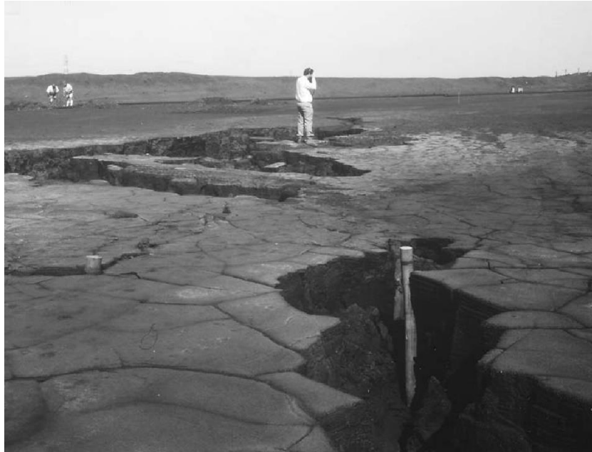
Figure 2.6: Example of erosion in shrinkage cracks following a storm on a paste tailings facility (Blight, 2010).
