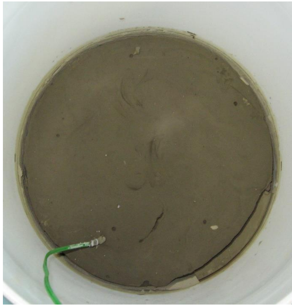
Figure 3.10: Examples of cracks in SL-01, ten days after deposition.
