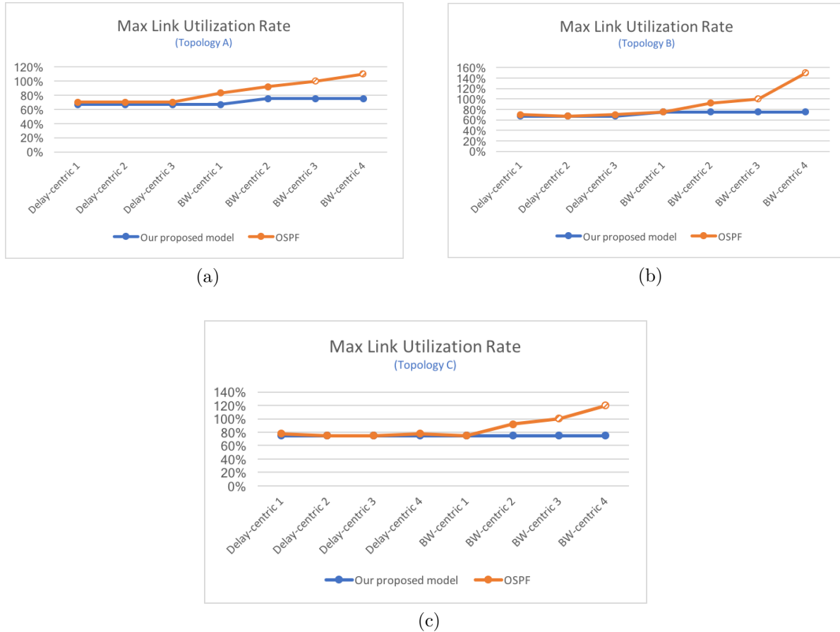
Figure 5.5 Maximum link utilization rate in the calculated paths by the proposed model and OSPF
