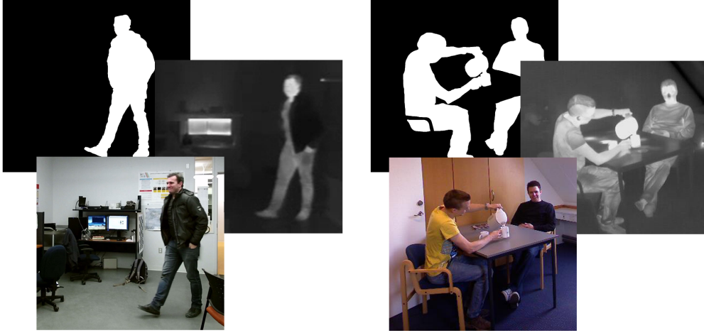
Figure 7.1 Examples of mutual foreground segmentation in low contrast conditions for RGB-LWIR image pairs. On the left, the person is only partly perceptible in the LWIR spectrum due to a winter coat, but is clearly perceptible in the visible spectrum. The opposite is true on the right, where legs are hard to perceive in the visible spectrum, but easy to perceive in the LWIR spectrum.
