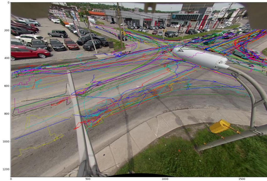
Figure 4.20: Illustration of the occlusion for the Jean-Proulx initial intersection camera view (view from the South approach)
