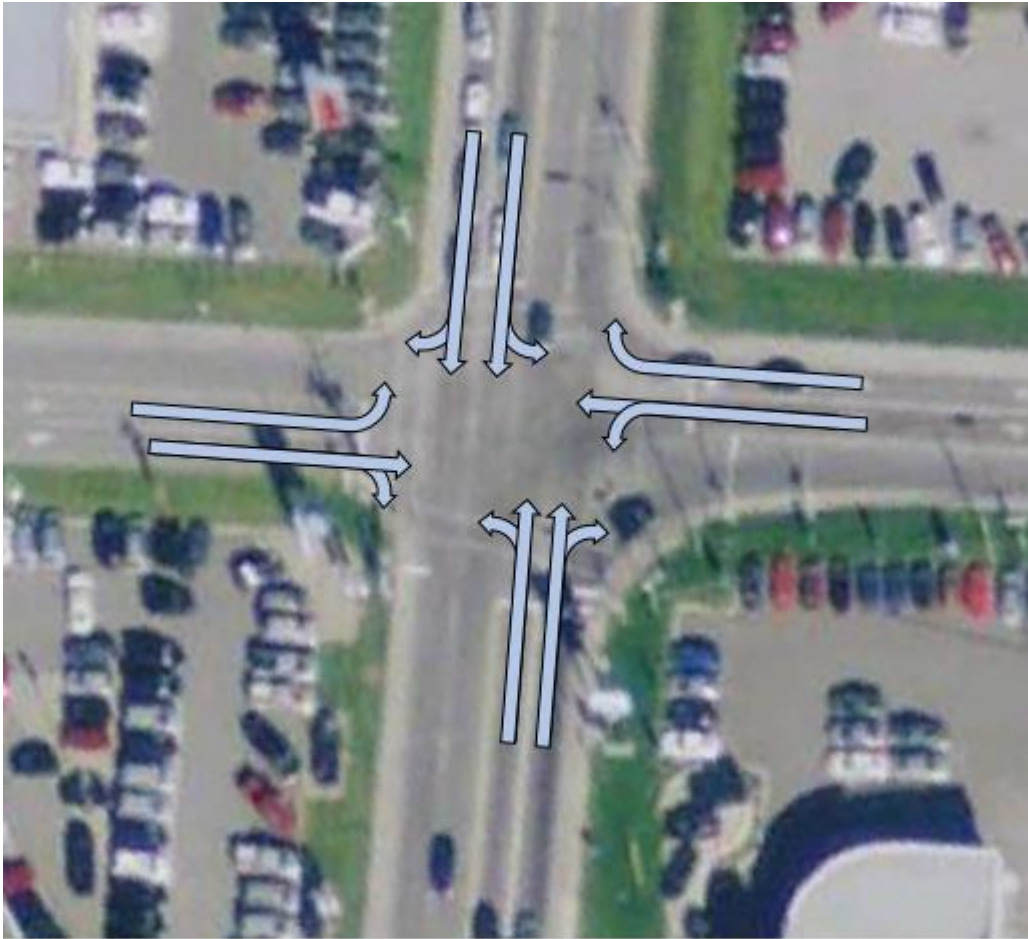
Figure 4.14: Satellite image of the Jean-Proulx intersection prior to roundabout conversion with allowed movements for each approach (Source: Google Earth, 2012)
