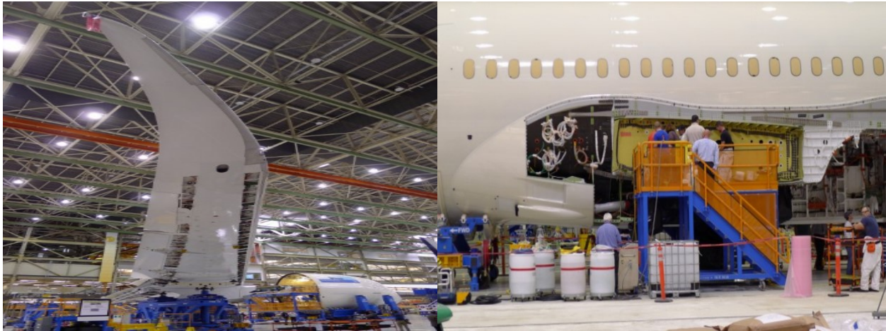
Figure 2-8: Assembling of the Boeing 787 Dreamliner; CFRP/Ti stack is used in the wing-fuselage connection (Paur, 2009, February 13)
