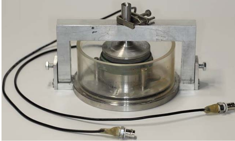
Figure 5-4: P-RAT implemented in an oedometer.
