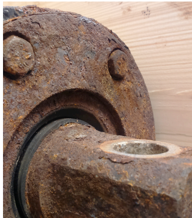
Figure 1.1: Part of a crank component of a Pelton turbine after service in a corrosive environment.
