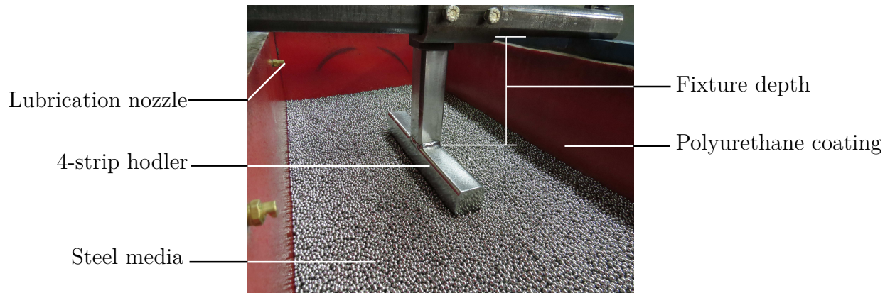
Figure 4.4 4-strips holder, flush with media surface
