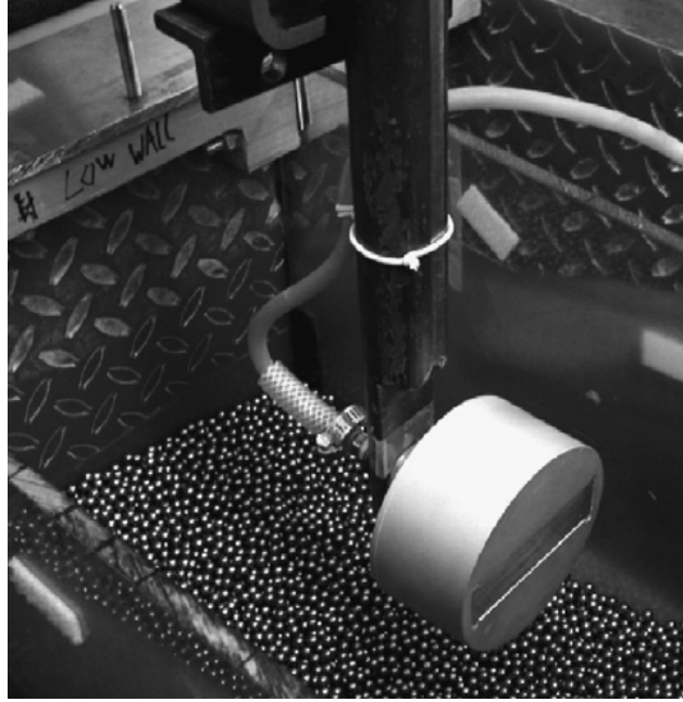
Figure 2.6 Picture of a strip holder inside the VP machine filled with steel media [23]
