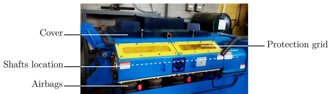
Figure 4.6 Actual vibratory peening machine, running with cover
