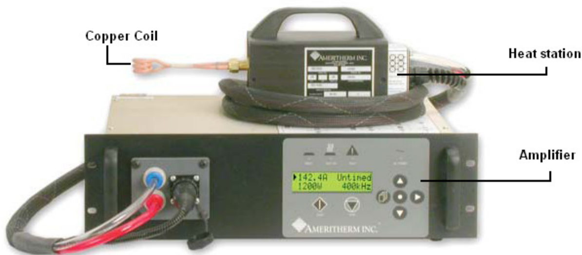
Figure 3.2. Ameritherm Inc TM HotShot 2kW induction heating
