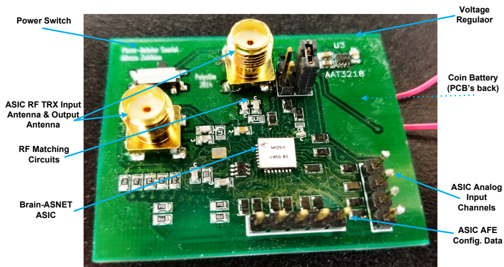
Figure 4.13: A Brain-ASNET sensor node module implemented using the fabricated ASIC
