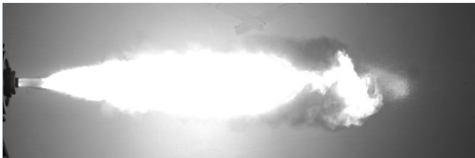
Figure 7.2: Reference propellant vented vessel flash
