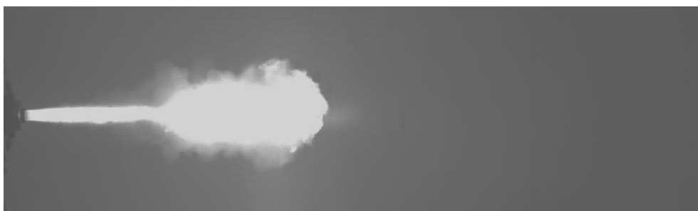
Figure 7.4: 35% HBT propellant vented vessel flash
