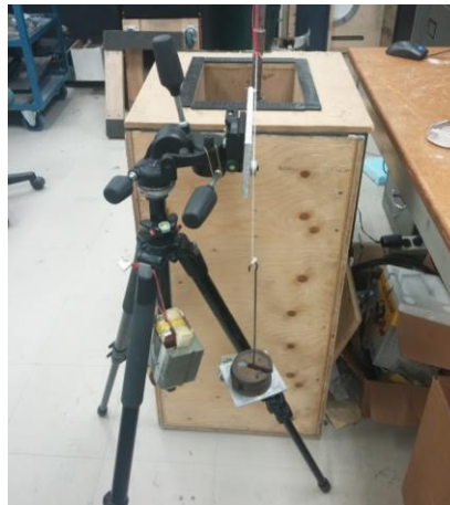
Figure 3-21 Calibration setup for L-shaped force balance
