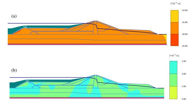
Figure 5-2: Horizontal (a) and vertical (b) deformations of the Franklin Falls Dam subjected to the 1988 Saguenay earthquake (record S16).
