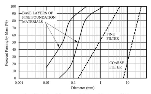
Figure 2-7: Grading of filter test materials (adapted from Brown, 1941)
