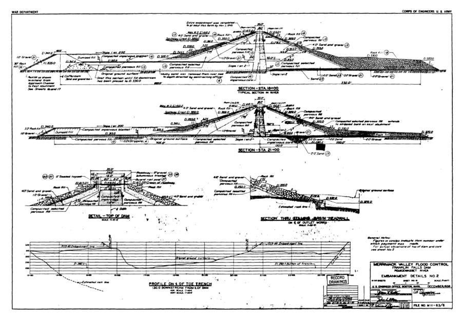
Figure A-2: Embankment details No.2
