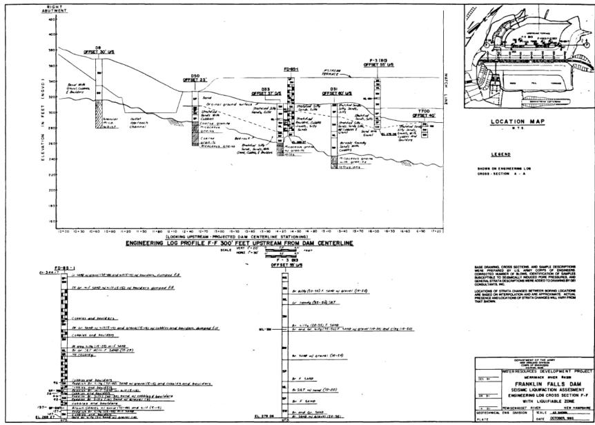
Figure A-8: Engineering log cross section F-F
