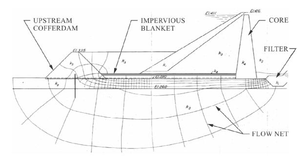
Figure 2-6: Flow net of the Franklin Falls dam with impervious blanket (USACE 1938).
