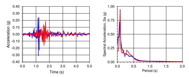
Figure 4-16: Recorded (blue) and estimated (red) transverse ground motions at the crest, and the corresponding spectral acceleration diagrams for 5% damping.
