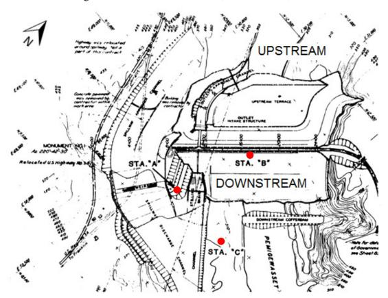
Figure 4-4: Plan view of the Franklin Falls Dam and location of accelerographs A, B and C (Chang 1987).
