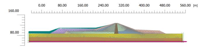
Figure 4-13: Finite element model of the Franklin Falls Dam used in PLAXIS 2D.
