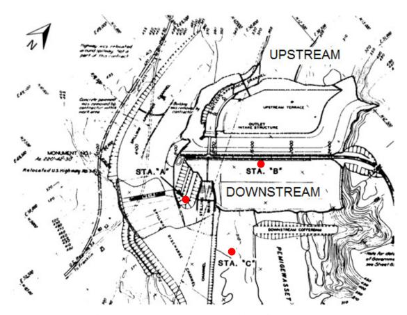
Figure 2-23: Plan view of the Franklin Falls Dam and location of accelerographs A, B and C (Chang 1987).
