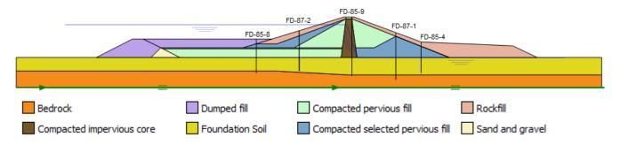
Figure 4-12: Cross section of the Franklin Falls Dam at station 18+00 used in PLAXIS.
