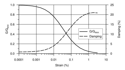
Figure 4-9: Shear damping ratios for sands at a mean effective stress of 100 kPa (Darendeli 2001).
