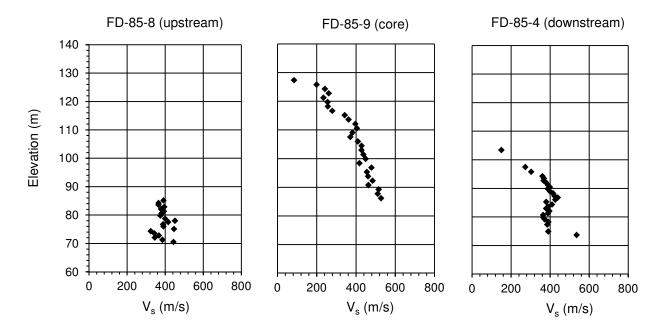
Figure 4-14: Estimated shear wave velocity profiles at Borehole FD-85-4, FD-85-9, and FD-85-4.
