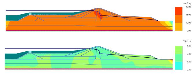
Figure 4-17: Horizontal (top) and vertical (bottom) deformations of the Franklin Falls Dam.
