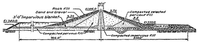
Figure 2-9: Typical cross-section of the dam (Brown 1941).
