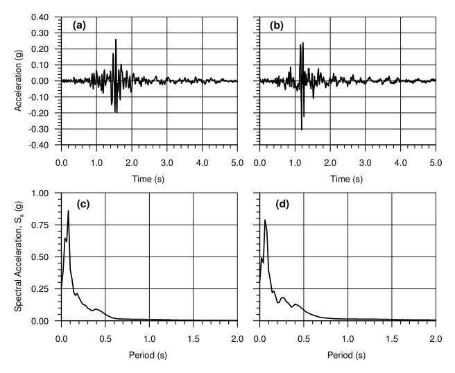
Figure 4-5: Measured transverse ground motions at the (a) downstream and (b) crest, and the corresponding spectral acceleration diagrams for 5% damping (c, d).
