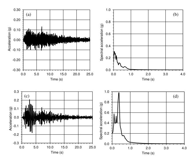
Figure 5-1: Ground motion (a) and spectral acceleration diagram (b) for 5% damping of Saguenay ground motion S16 (Transverse); Calculated ground motion (c) and special acceleration diagram for 5% damping (d) at crest of dam.
