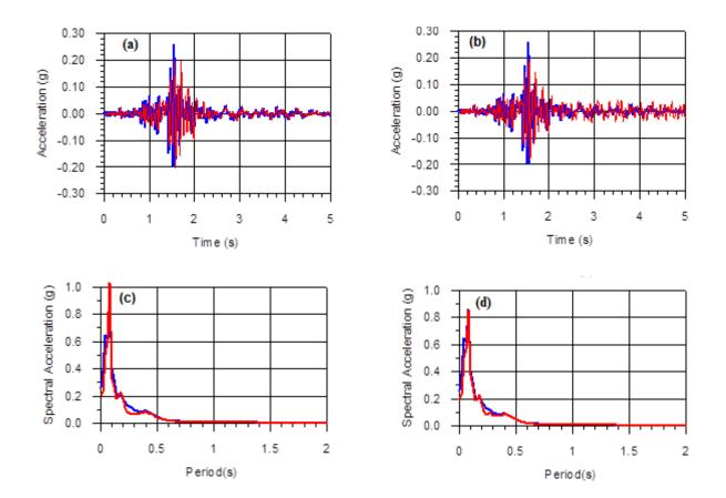
Figure 4-11: Measured transverse ground motions (blue) compared to generated ground motions (red) using (a) Rayleigh damping and (b) Hysteretic damping, and the corresponding spectral acceleration diagrams for 5% damping (c, d) (St-Michel and James 2017).
