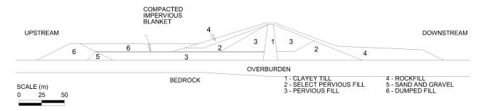
Figure 4-3: Typical cross section of Franklin Falls Dam (James and Arbaiza 2015).
