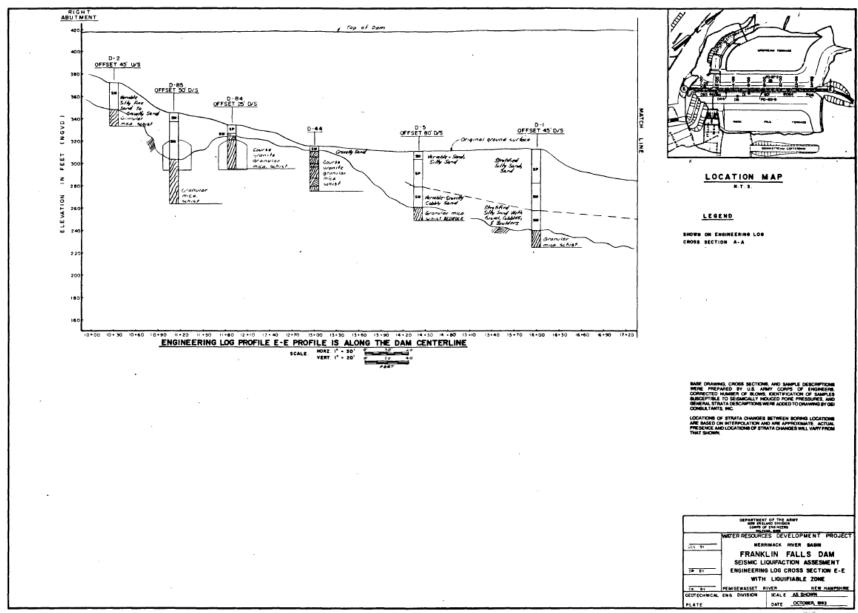
Figure A-7: Engineering log cross section E-E
