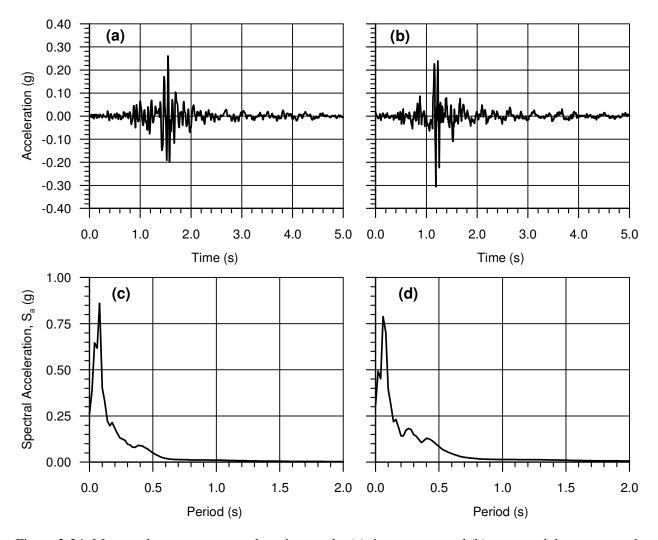
Figure 2-24: Measured transverse ground motions at the (a) downstream and (b) crest, and the corresponding spectral acceleration diagrams for 5% damping (c, d) (James and Arbaiza 2015).
