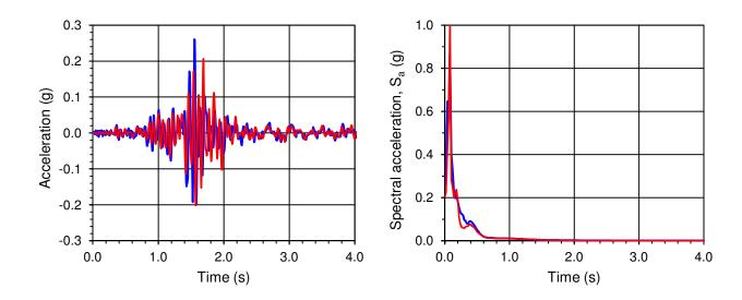
Figure 4-10: Measured transverse ground motion (blue) compared to generated transverse ground motion (red) and spectral acceleration diagram for 5% damping at the downstream accelerograph.
