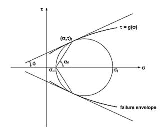
Figure 2-27: Mohr diagram and failure envelope (Plaxis 2010).
