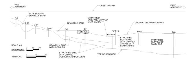
Figure 4-2: Longitudinal cross section of subsurface conditions (James and Arbaiza 2015).
