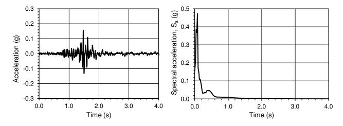
Figure 4-6: Calculated transverse ground motion on bedrock and spectral acceleration diagram for 5% damping at the downstream accelerograph (James and Arbaiza 2015).
