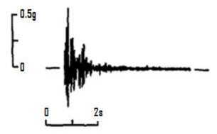
Figure 2-18: Acceleration of the 1982 Miramichi earthquake at station Loggie Lodge (Bhan and Dunbar 1989).
