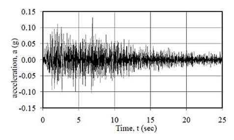
Figure 2-22: Ground motion of the 1988 Saguenay earthquake at station S16 (NRC, 2003).
