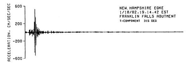
Figure 2-20: Transversal acceleration of the 1982 Gaza earthquake at the abutment of the Franklin Falls Dam (Chang 1983).
