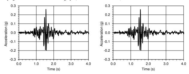
Figure 4-7: Measured (left) and calculated (right) transverse ground motion at the downstream accelerograph.
