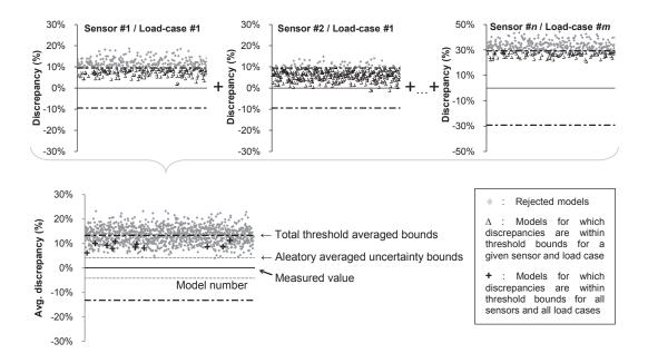
FIGURE 8 - CANDIDATE MODEL SELECTION PROCESS USING THRESHOLD
