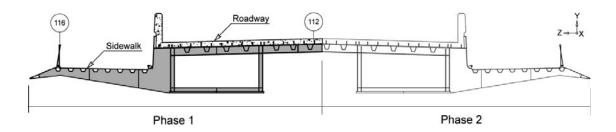
FIGURE 3 – CONSTRUCTION PHASES OF LANGENSAND BRIDGE
