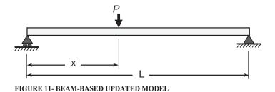
Measurements from one load case are used to compute the equivalent flexural stiffness of the bridge. Using the four measurements and equations (2) and (3), the average flexural stiffness is evaluated. One of the results are presented in Table 4.
