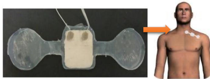
Figure 2.20: Photograph of sensor patch (transparent = PDMS and opaque = PVDF) [117]
