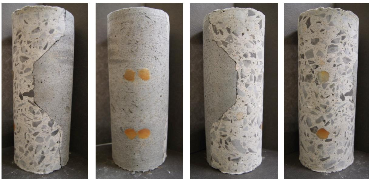
**Figure I- 10 : Carotte – Dalle 12' (2o-D-C-1-F) – Avant rupture [SO]**
