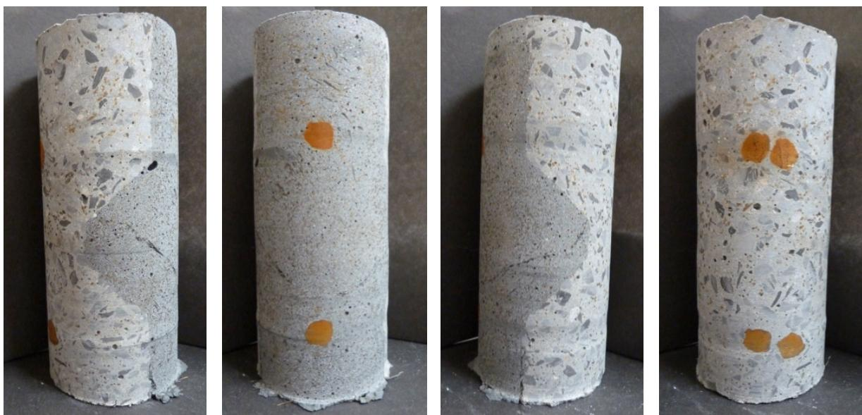
**Figure I- 24 : Carotte – Dalle 22' (2f-U-Q-1-F) – Avant rupture [SO]**
