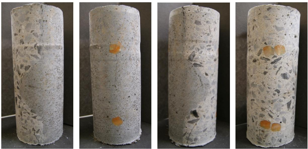
**Figure I- 21 : Carotte – Dalle 20' (3o-U-Q-1-F) – Avant rupture [SO]**
