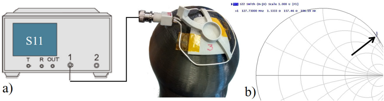
Figure 4.36 Impedance measurement setup to find the loop inductance (a) and one result (b).
