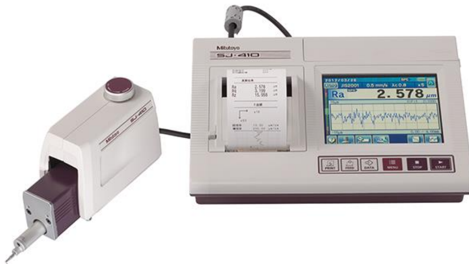
Figure 3.9: Surface roughness tester SJ-410, Mitutoyo ( www.mitutoyo.com )
