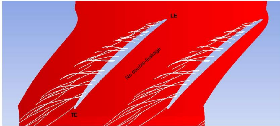
Figure 5.19: Double-leakage extent at the rotor tip plane at nominal tip clearance in the presence of the final casing treatment
