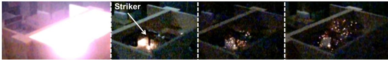
Figure 5.11: Snapshots from 40 kA lightning impulse strike on Cu\Sn continuous coatings showing hot runaway coating fragments
