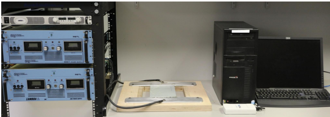
Figure 7.3: Key electrical equipment for continuous current emulation
