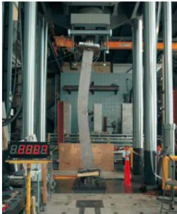
Figure 2.9: Column specimen at the end of test (Lamarche and Tremblay 2011).
