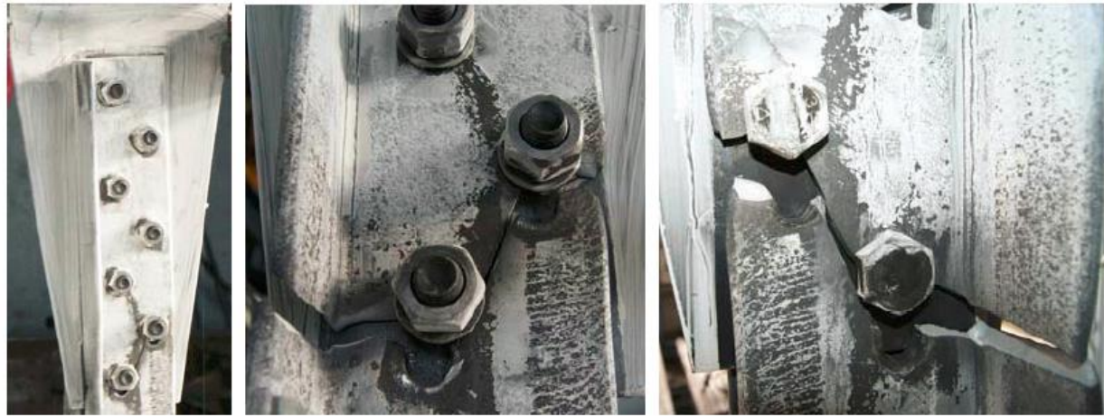
Figure 7.2: Failure in brace connection (Tremblay et al. 2012).
