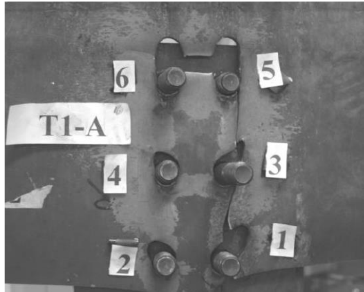
Figure B.9: Block shear failure of a bolted gusset plate (Singh Huns et al. 2002).
