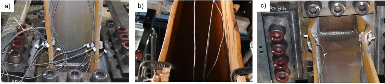
Figure A.22: Local buckling of specimen CS7 at a) bottom; b) middle; and c) top of column.
