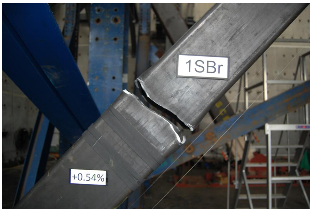
Figure 1.1: Brace fracture of NCFB specimen (Sen et al. 2016a).
