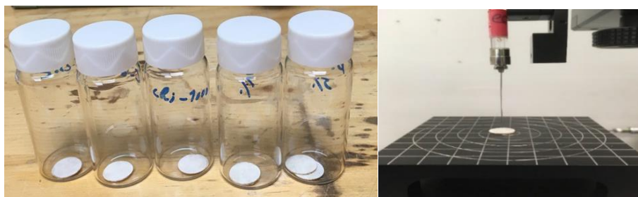
Figure 3.6. Prepared samples for contact angle measurements.
