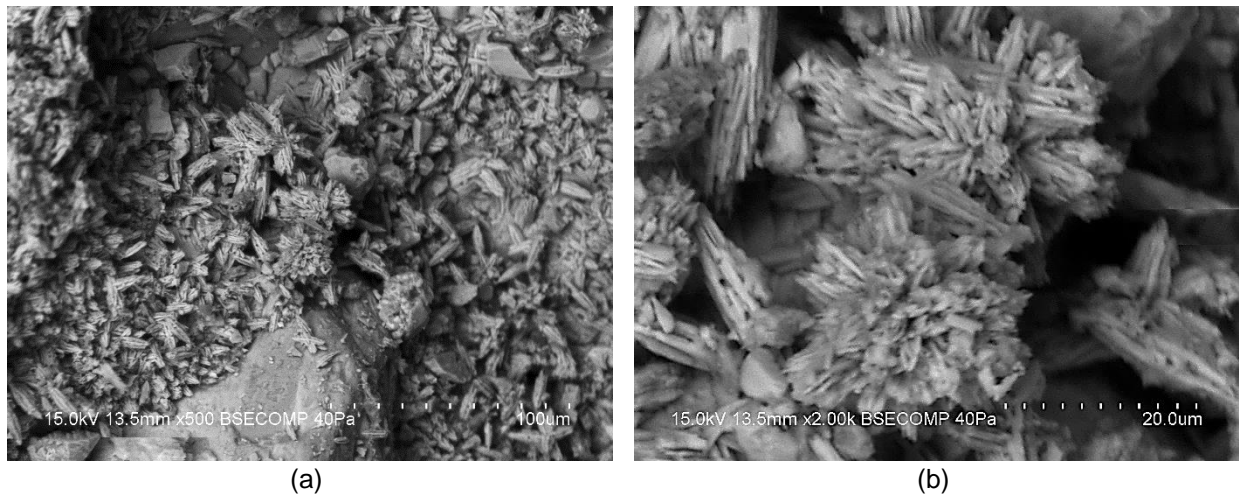
Figure 5-12 : SEM observation of the self-healing products in HPFRC-CA cracks
