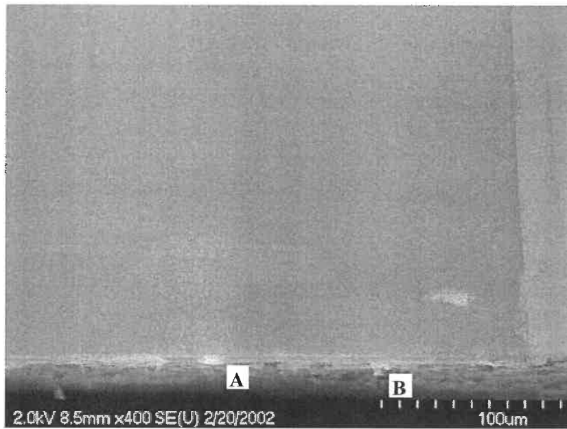
Figure 4.54: Low magnification view indicating a relatively constant width of the deformation zone (crack propagation direction is horizontal; references A and B for the next figures).
