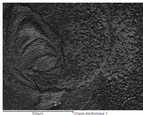
Figure 5.17: Area 5 (broad region) near the center of the Ni sealing (Figure 5.7). Average composition of the entire region: \text{NiF}_2 +NiO (major phases), Ni-Cu alloy (minor phase), Fe+Ti+C (traces).
