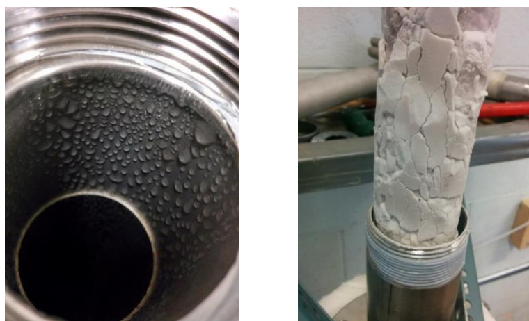
Figure 4.8: Condensation of water at the outlet of HTFB at temperatures higher than 500°C causing the particles to stick to the filter.
