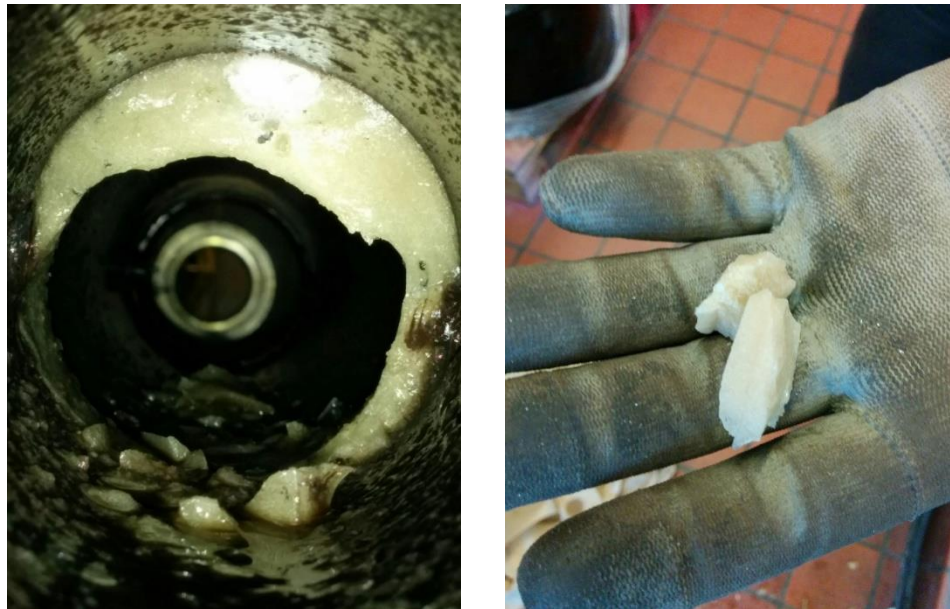
Figure 4.14: Formation of hard agglomerates of GB71 after full defluidization at 500°C.
