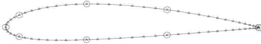
(a) Geometric form comparison with 9 control points between the parametric and original airfoils
