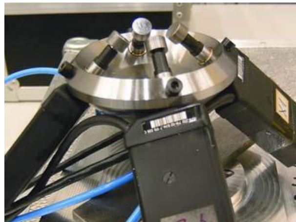
Figure 2.7: left: Schematic configuration of the pseudo-3D-artefact; right: linear displacement measurement system with four sensors (Bringmann et al., 2005)
