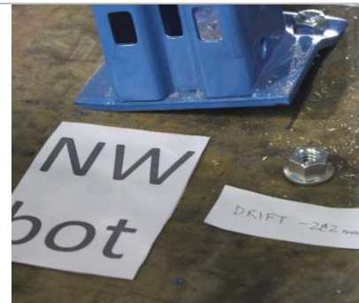
Figure B-3 : Typical damage to base plate test F1
