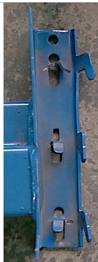
Figure B-33 : Typ. Connector after test
