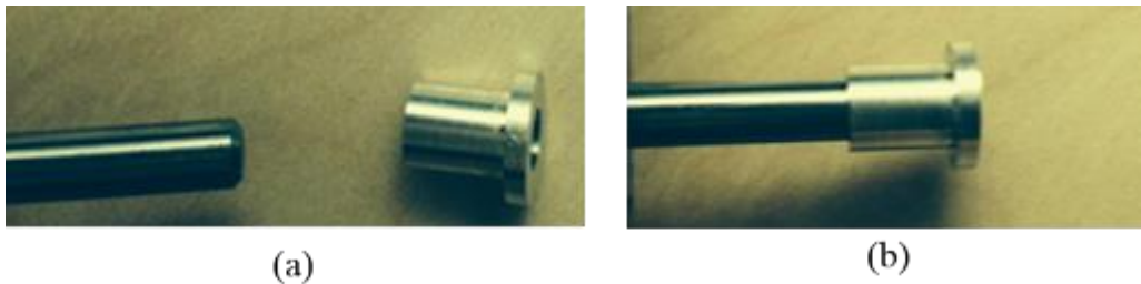
Figure 3.21 Increase the shaft area at its end.
