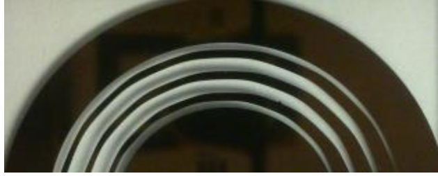
Figure 3.6 Fabricated mask with polylines instead of curves.
