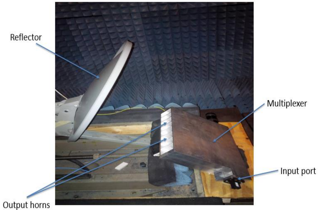
Figure 5-1: Picture of the parabolic dish fed by the frequency beam scanning system [12].
