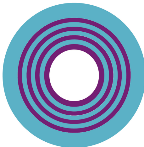
Figure 1.1 A Bragg fiber featuring a large hollow core surrounded by a periodic sequence of high and low refractive index layers.
