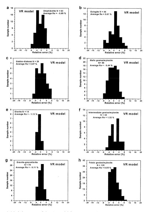
Figure 3.6 Relative errors of the VR model for 15 common lithologic categories. Calculated Vp data are compared with measured values at 300 MPa. N – Sample number. The relative error is defined by Equation (3.2).
