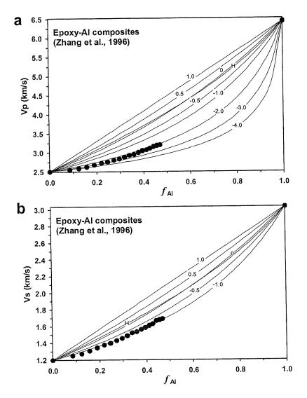
Figure A1.12 P-wave (a) and S-wave (b) velocities for epoxy-Al composites plotted against volume fraction of Al. Theoretical curves labelled according to J value. H represents the Hill average.
