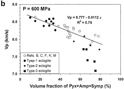
Figure 4.9 Variations of eclogite P-wave velocity at 600 MPa as a function of (a) garnet (Grt) content and (b) the volume fraction of pyroxene (Pyx), amphibole (Amp) and symplectite (Symp). Unaltered eclogites from references are also plotted. Abbreviations for references: B – Birch (1960), C – Christensen (1974), F – Fountain et al. (1994), K – Kern et al. (1999, 2002), M – Manghnani et al. (1974). Solid line is the least squares fit to data, excluding Type-3 eclogites.
