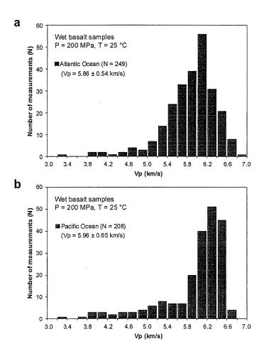
Figure 2.4 Histogram of P-wave velocities at 200 MPa and 25 °C of wet basalt samples from (a) Atlantic Ocean and (b) Pacific Ocean.
