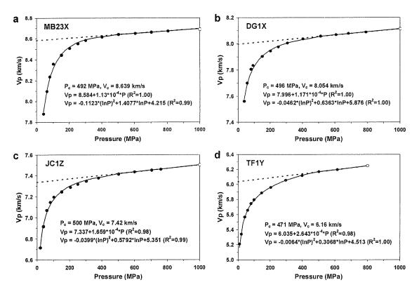
Figure 4.12 Experimental data points are best fit by the expressions  $V = a(\ln P)^2 + b \ln P + c$  and  $V = DP + V_0$  at pressures below and above  $P_c$ , respectively. (a) Core X from MB23 (Type-1 eclogite), (b) Core X from DG1 (Type-2 eclogite), (c) Core Z from JC1 (Type-3 eclogite), and (d) Core Y from TF1 (granitic gneiss).
