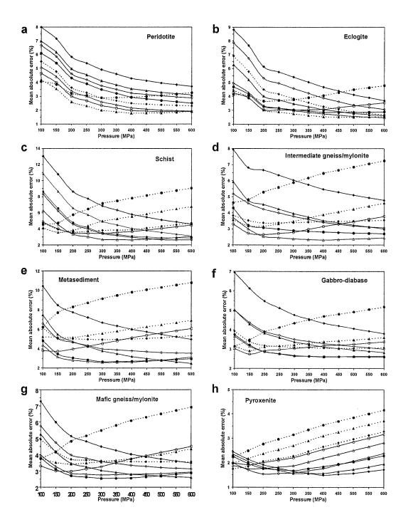
Figure 3.3 Comparison of the theoretical P-wave velocities (zero porosity, 25 °C and 0.1 MPa) with those measured at different pressure for 15 common categories of rocks. Mean absolute error  $(\overline{Ae}, \%)$  is taken as a statistic measure of the goodness of each averaging model.
