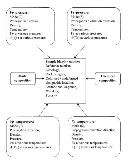
Figure 2.1 Structure of the database of rock seismic properties (DRSP).
