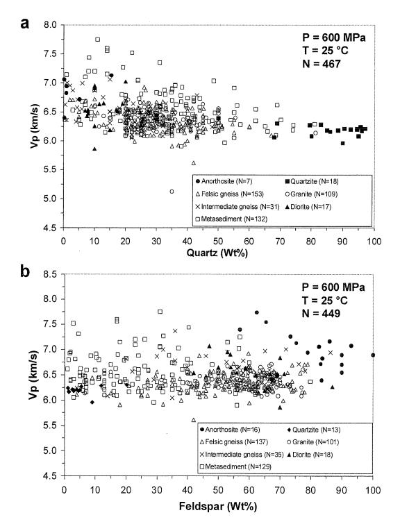
Figure 2.11 P-wave velocities at 600 MPa of quartzofeldspathic rocks versus (a) quartz content and (b) feldspar content. N- Sample number.
