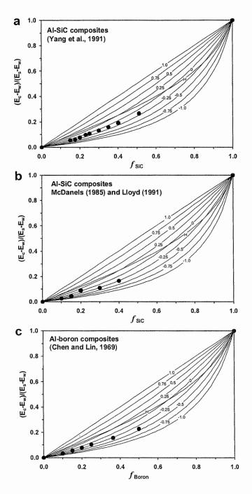
Figure A1.7 Theoretical curves on relative Young's modulus  $(E_c-E_m)/(E_s-E_m)$  for aluminium-matrix composites plotted against volume fraction of reinforcement. Al-SiC composites (a and b) and Al-boron composites (c). *J* value is given in number. H represents the Hill average.
