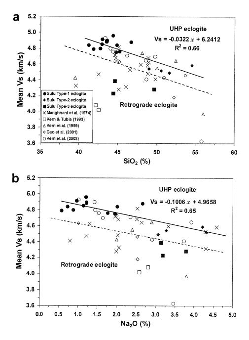
Figure 5.5 Chemical dependence of shear wave velocities at 600 MPa of eclogites: (a)  $\overline{V}s$ -SiO<sub>2</sub> content, (b)  $\overline{V}s$ -Na<sub>2</sub>O content. The dashed line separates UHP eclogites and retrograde eclogites, while the solid line represents the least squares fit to the data for Type-1 and Type-2 eclogites from Sulu.
