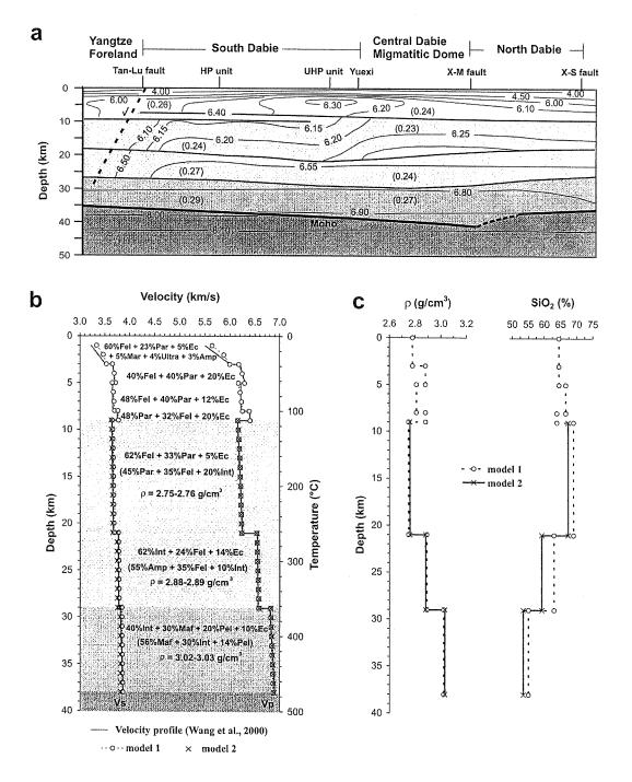
Figure 5.16 (a) Seismic refraction profile BB' across the Dabie Mountains (see Figure 5.1) with Vp and Poisson's ratios in parentheses (after Wang et al., 2000), X-M fault: Xiaotian-Mozitan fault; X-S fault, Xinyang-Shucheng fault. (b) Inferred crustal composition beneath the Dabie UHP unit. Lithology symbols are defined in Figure 14b. (c) Density and SiO<sub>2</sub> content with depth, calculated using Model 1 and Model 2.
