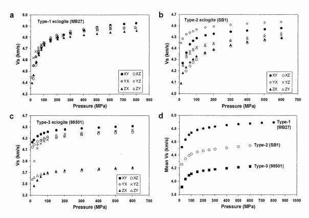
Figure 5.2 Plot of shear wave velocity (*Vs*) versus confining pressure for three typical types of eclogites: (a) Type-1 eclogite MB27, (b) Type-2 eclogite SB1, (c) Type-3 eclogite 98501, and (d) mean shear wave velocities of these three samples.
