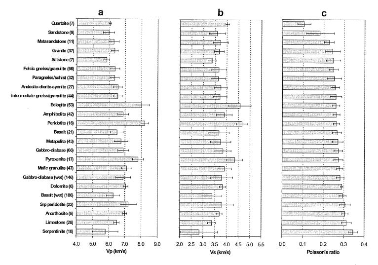
Figure 2.17 Average seismic velocities and Poisson's ratios at 600 MPa of common rock types. (a) Vp, (b) Vs and (c) Poisson's ratio. Error bars represent  $2\sigma$  standard deviations of the datasets. The sample number of each rock type is given in parentheses.
