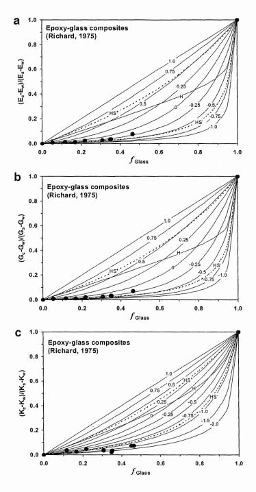
Figure A1.10 Comparison of the predictions of the present approach, the Hashin-Shtrikman upper  $(HS^{+})$  and  $(HS^{-})$  bounds with experimental data on relative Young's modulus (a), shear modulus (b) and bulk modulus (c) of epoxy-glass composites. J value is given in number. H represents the Hill average.
