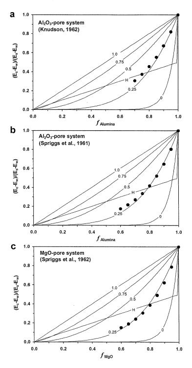
Figure A1.1 Experimental and theoretical results for relative Young's modulus of porous  $Al_2O_3$  (a and b) and MgO (c) as a function of the volume fraction of solid component. Curves labelled according to J value. H represents the Hill average.
