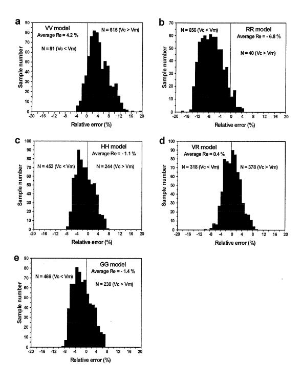
Figure 3.4 Relative errors of the VV (a), RR (b), HH (c) and VR (d) models for 696 samples. Calculated Vp data ( $V_c$ ) are compared with measured values ( $V_m$ ) at 300 MPa. N – Sample number. The relative error is defined by Equation (3.2).
