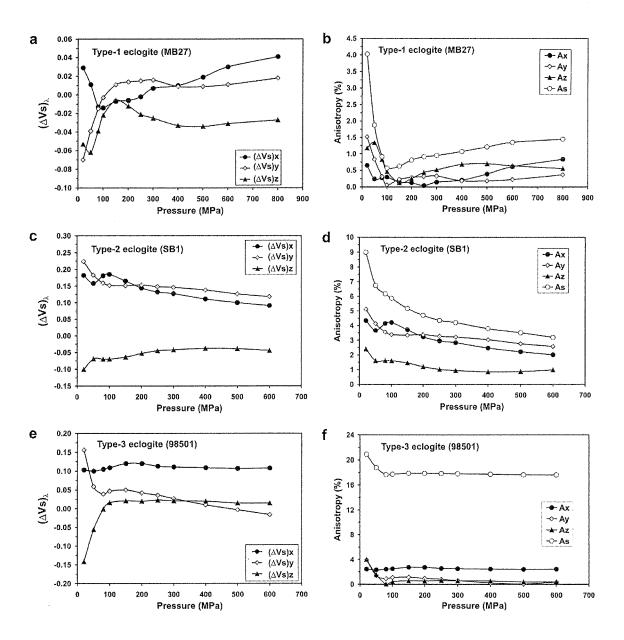
Figure 5.7 Pressure dependence of shear wave splitting ( $\Delta Vs$ ), splitting-produced anisotropy ( $A_{\lambda}$ ) along a given propagation direction  $\lambda$  (X, Y or Z) and bulk anisotropy (As) for (a-b) Type-1 eclogite MB27, (c-d) Type-2 eclogite SB1 and (e-f) Type-3 eclogite 98501, respectively.
