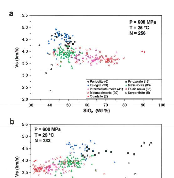
Figure 2.13 (a) Vs versus SiO<sub>2</sub> content at 600 MPa and 25°C for 255 samples, and (b) Vs versus content of Fe<sub>2</sub>O<sub>3</sub>+FeO+MgO at 600 MPa and 25°C for 234 samples. The sample number of each rock type is given in parentheses.
