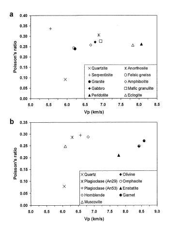
Figure 1.5 Comparison of (a) measured Poisson's ratio and Vp (200 MPa, 25 °C) of common rock types with (b) theoretical values of monomineralic aggregates (zero porosity, 0.1 MPa and 25 °C).
