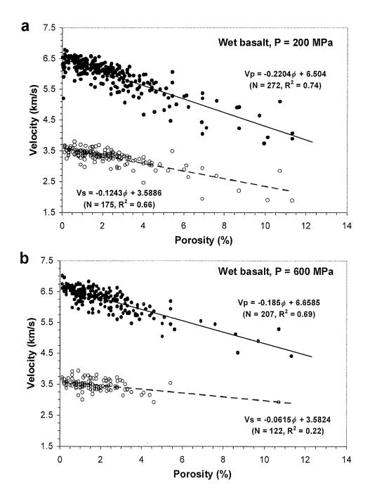
Figure 2.10 Dependence of P- and S-wave velocities on porosity  $(\phi)$  of water-saturated basalts at confining pressure of (a) 200 MPa and (b) 600 MPa. N is the sample number; solid line and dashed line are the least squares fit to Vp data (solid circle) and Vs data (open circle), respectively.
