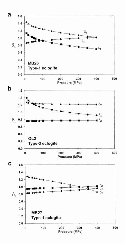
Figure 4.15 Normalized pressure derivative  $(\delta_{\lambda})$  as a function of pressure in the nonlinear regime for (a) Pattern 1, (b) Pattern 2, and (c) Pattern 3 anisotropy (see text).
