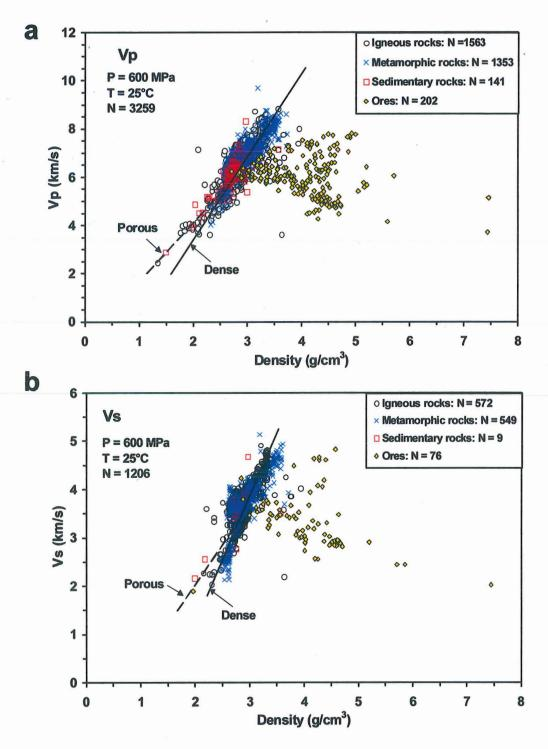
Figure 2.6 (a) Vp-density and (b) Vs-density relations at 600 MPa and 25 °C.
