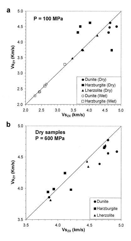
Figure 2.16 Split shear wave velocities of peridotites along Z-direction at (a) 100 MPa and (b) 600 MPa. The diagonal indicates zero shear wave splitting.
