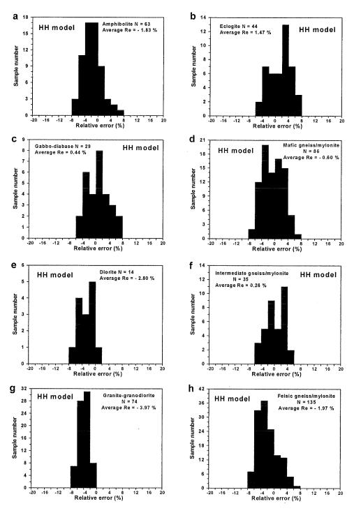
Figure 3.5 Relative errors of the HH model for 15 common lithologic categories. Calculated Vp data are compared with measured values at 300 MPa. N – Sample number. The relative error is defined by Equation (3.2).
