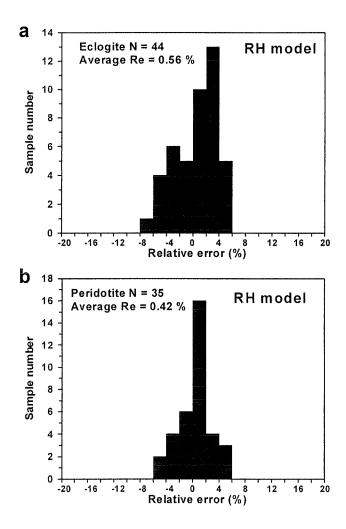
Figure 3.7 Relative errors of the RH model for eclogite (a) and peridotite (b). Calculated Vp data are compared with measured values at 300 MPa. N – Sample number. The relative error is defined by Equation (3.2).
