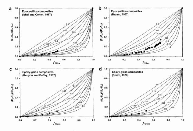
Figure A1.9 Comparison of the predictions of the present approach, the Hashin-Shtrikman upper (HS<sup>+</sup>) and lower (HS<sup>-</sup>) bounds, Paul's (1960) calculations (P) with experimental data on relative elastic Young's moduli of epoxy resin-based composites. Epoxy-Silica composites (a and b) and epoxy-glass composites (c-d). *J* value is given in number. H represents the Hill average.
