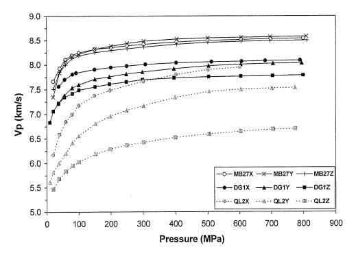
Figure 4.7 P-wave velocities versus pressure in the X, Y and Z directions for three typical eclogite samples (MB27: Type-1 eclogite; DG1: Type-2 eclogite; QL2: Type-3 eclogite) from the Sulu UHP zone.
