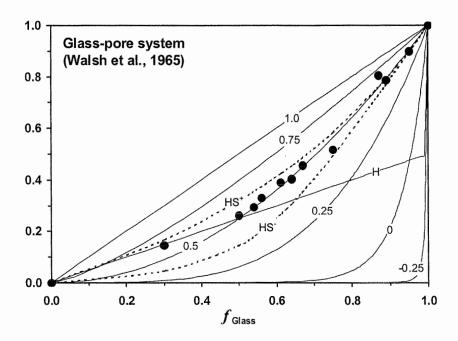
Figure A1.2 Comparison between experimental and theoretical results for relative bulk modulus (Kc-Kw)/(Ks-Kw) for glass foams. Theoretical curves labeled according to J value. H, HS+ and HS- represent the Hill average, the Hashin-Shtrikman upper and lower bounds, respectively.
