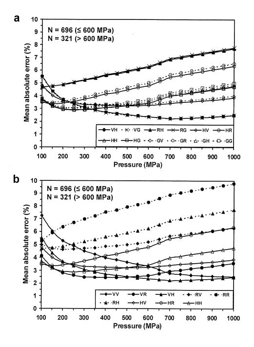
Figure 3.1 Comparison of the theoretical P-wave velocities (zero porosity, 25 °C and 0.1 MPa) with those measured at different pressure. Mean absolute error ( $\overline{Ae}$ , %) is taken as a statistic measure of the goodness of each averaging model. N – Sample number.
