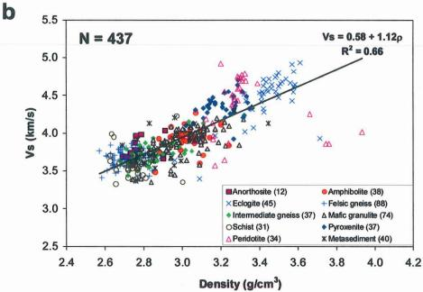
Figure 2.7 (a) *Vp*-density and (b) *Vs*-density relations for typical lower crustal rocks measured at 600 MPa and 25 °C. N – Sample number. The number in parentheses is the sample number of each lithology.
