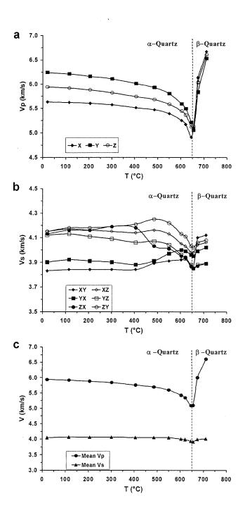
Figure 1.6 Variations of seismic properties at 600 MPa in a quartzite due to the  $\alpha$ - $\beta$  quartz transition with changing temperature. (a) P-wave velocities in the X, Y and Z directions, (b) S-wave velocities propagating and vibrating in the X, Y, and Z directions, and (c) the mean P- and S-wave velocities. After Ji et al. (2002) and original experimental data from Barruol (1993).
