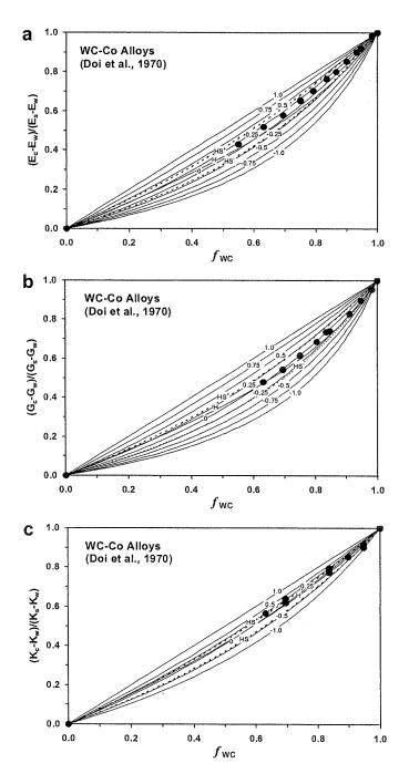
Figure A1.5 Relative Young's modulus (a), shear modulus (b) and bulk modulus (c) for WC-Co alloys plotted against volume fraction of WC. Theoretical curves labeled according to J value. H,  $HS^+$  and  $HS^-$  represent the Hill average, the Hashin-Shtrikman upper and lower bounds, respectively.
