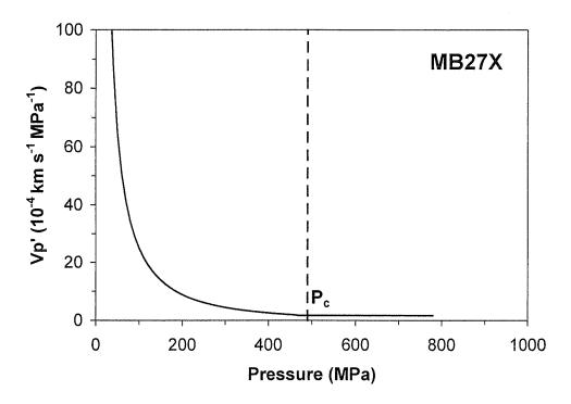
Figure 4.13 Pressure derivative (Vp') as a function of pressure for Sulu eclogite MB27X.  $P_c$  is the critical pressure above which microcracks and pores are closed and the sample behaves as a compacte aggregate.
