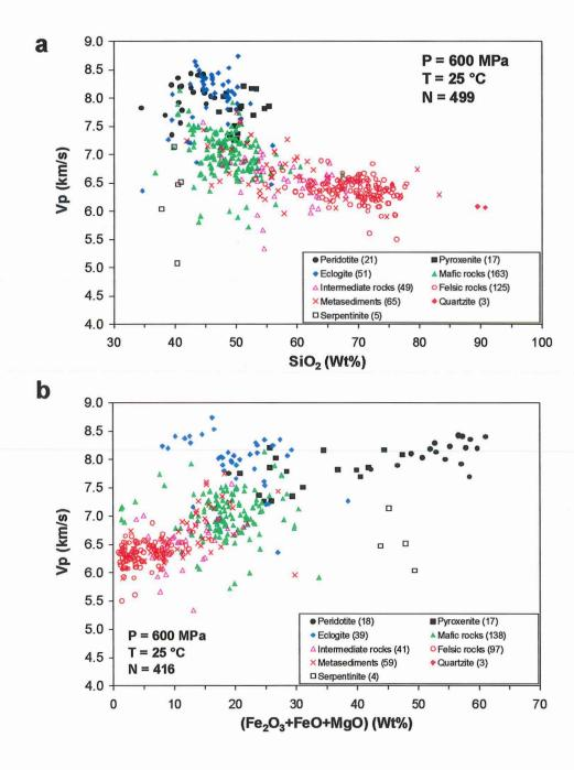
Figure 2.12 (a) Vp versus SiO<sub>2</sub> content at 600 MPa and 25°C for 499 samples, and (b) Vp versus content of Fe<sub>2</sub>O<sub>3</sub>+FeO+MgO at 600 MPa and 25°C for 416 samples. The sample number of each rock type is given in parentheses.
