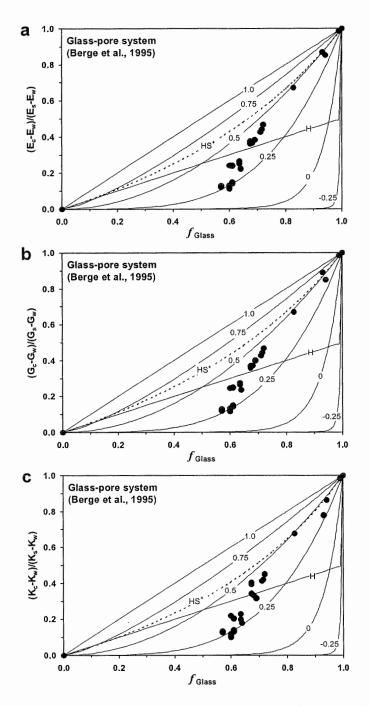
Figure A1.3 Comparison between experimental and theoretical results for relative Young's modulus (a), shear modulus (b) and bulk modulus (c) for sandstone analogs made from fused glass beads. Theoretical curves labeled according to J value. H and  $HS^+$  represent the Hill average and the Hashin-Shtrikman upper bound, respectively.
