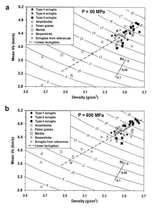
Figure 5.3 Mean shear wave velocities ( $\overline{V}s$ ) versus densities at (a) 50 MPa and (b) 600 MPa of Dabie-Sulu UHP rocks. The dashed line is the best-fit solution for  $\overline{V}s$  versus density for eclogites from this study and references. Also shown are lines of constant acoustic impedance and a floating reflection coefficient (Rc) scale.
