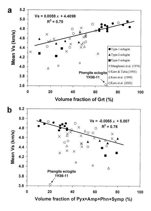
Figure 5.4 Mean shear wave velocities (*Vs*) of eclogites at 600 MPa versus volume fraction of (a) garnet (Grt) and (b) pyroxene (Pyx), amphibole (Amp), phengite (Phn) and symplectite (Symp). Solid line is the least squares fit to the data for Type-1 and Type-2 eclogites from the Sulu UHP metamorphic belt.
