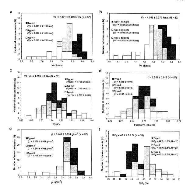
Figure 5.13 Histograms of petrophysical properties of eclogites: (a) P-wave velocity (Vp), (b) S-wave velocity (Vs), (c) Vp/Vs ratio, (d) Poisson's ratio, (e) density and (f) SiO<sub>2</sub> content. Vp, Vs, Vp/Vs ratio and Poisson's ratio are given at 600 MPa and room temperature. N: number of measurements.
