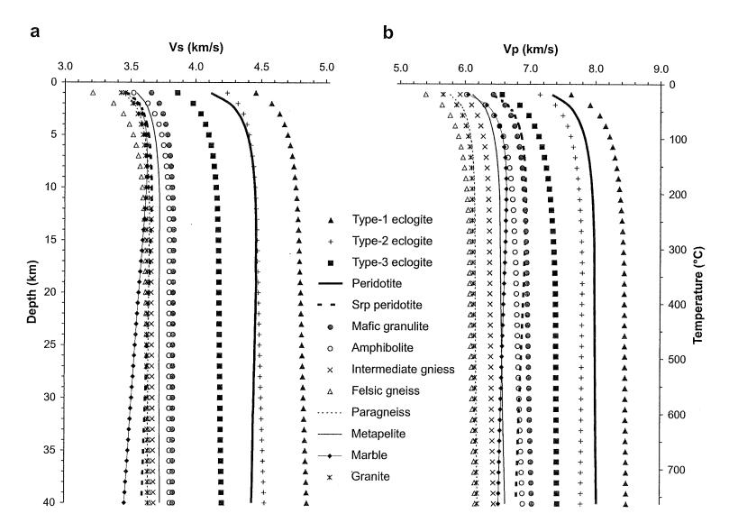
Figure 5.12 Calculated in situ (a) S-wave velocities and (b) P-wave velocities with depth for the Sulu crust.
