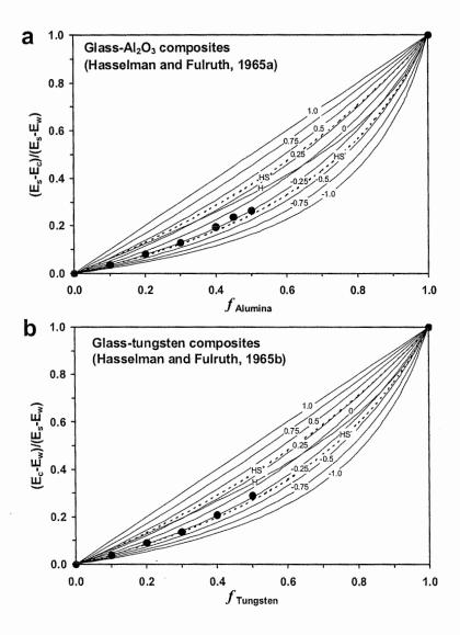
Figure A1.13 Theoretical curves on relative Young's modulus  $(E_c-E_w)/(E_s-E_w)$  for glass-matrix composites plotted against volume fraction of reinforcement. Glass-Al<sub>2</sub>O<sub>3</sub> composites (a) and glass-tungsten composites (b). Theoretical curves labelled according to J value. H, HS<sup>+</sup> and HS<sup>-</sup> represent the Hill average, the Hashin-Shtrikman upper and lower bounds, respectively.
