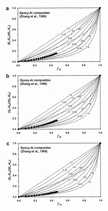
Figure A1.11 Relative Young's modulus (a), shear modulus (b) and bulk modulus (c) for epoxy-Al composite plotted against volume fraction of Al. Theoretical curves labeled according to J value. H,  $HS^+$  and  $HS^-$  represent the Hill average, the Hashin-Shtrikman upper and lower bounds, respectively.
