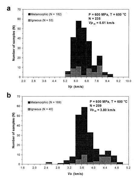
Figure 2.3 (a) Histogram of P-wave velocities for 235 samples, and (b) histogram of S-wave velocities for 209 samples at 600 MPa and 600 °C.
