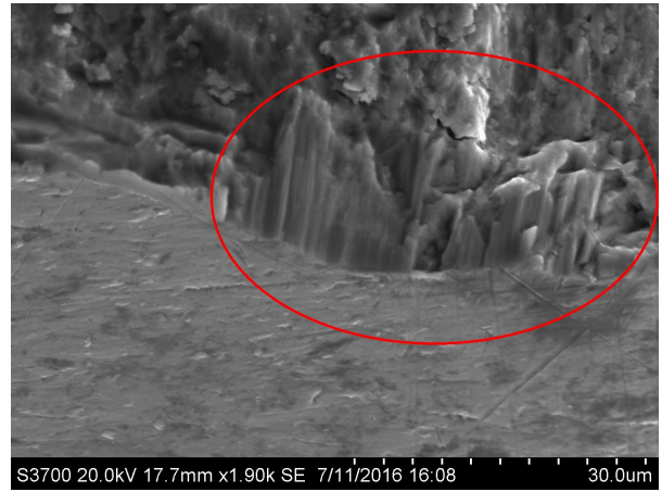
(b) Magnification of the red circled area in Figure 5.9a showing the \alpha colony where the crack nucleated. Note that the initiation site is circled for clarity
