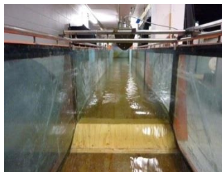
Figure 4.4. Flow over a triangular sill (left) – Second configuration, sectional view (right)
