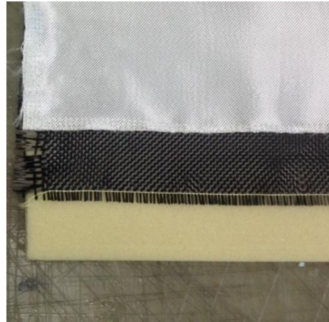
Figure 3-6: 7781 8H glass and 94101 plain 3k T-300 carbon Fibres fabrics and SAN core
