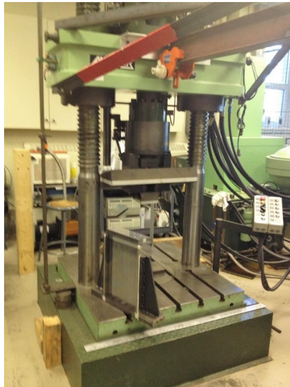
Figure 3-20: AMSLER 600-ton universal test machine
