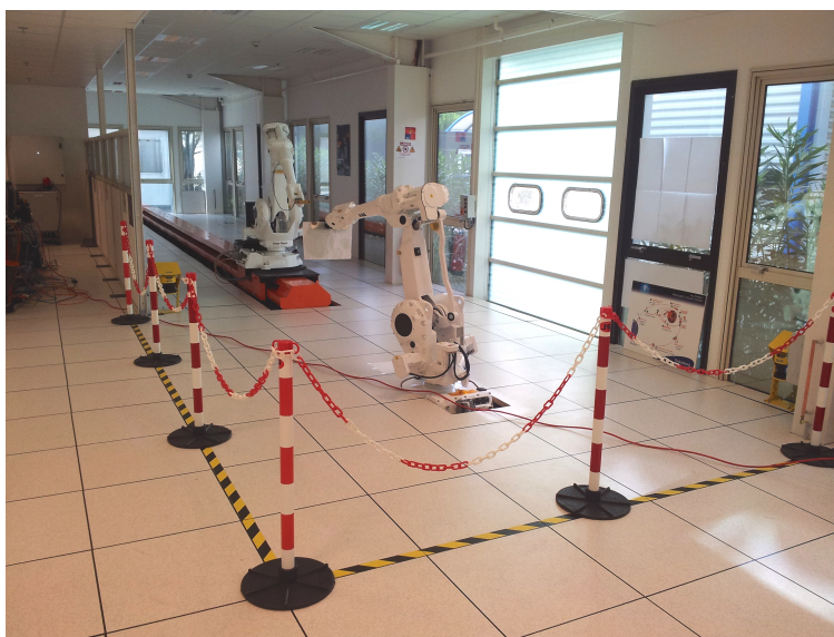
Figure 9.7: Robotic test bench used to simulate the on-orbit kinematics of a capture
