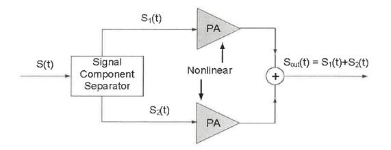
Figure 2.1 Basic schematic diagram of the LINC transmitter
