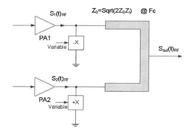
Figure 3.8 Variable reactive termination combiner
