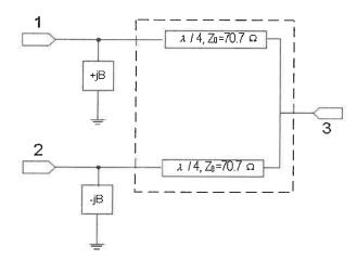
Figure 3.6 Chireix outphasing system with shunt susceptances
