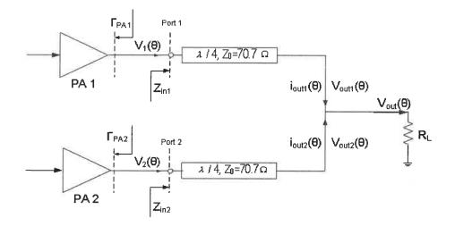
Figure 3.5 Lossless combiner analysis
