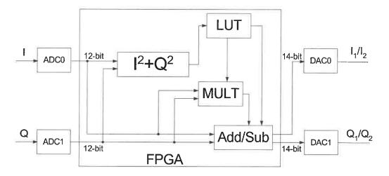
Figure 2.7 Method 1 --- LUT design block diagram
