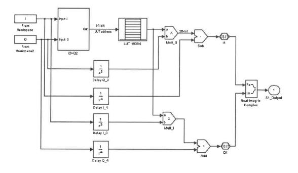
Figure 2. 14 Top level design for S<sub>1</sub> in Simulink ---- method 1 LUT
