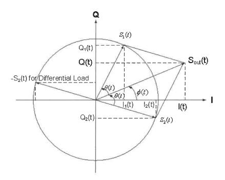
Figure 2.3 Vector diagram illustrating relationship between components
