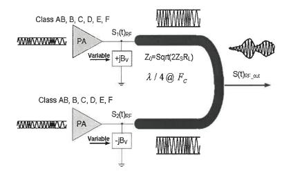
Figure 1.5 Variable reactive termination combiner
