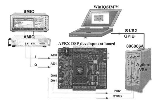
Figure 2. 21 Measurement set-up
