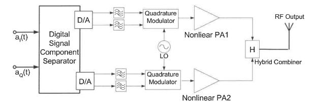
Figure 1.3 LINC transmitter with digital signal component separator
