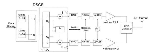
Figure 2.4 LINC implementation with a new DSCS architecture
