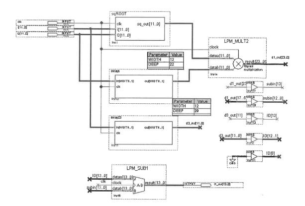
Figure 2.13 Top level design for  $I_1(n)$  with SRFB in the Quartus II 2.0
