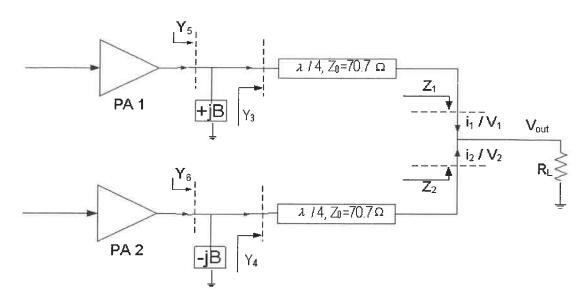
Figure 3.7 Chireix outphasing system analysis
