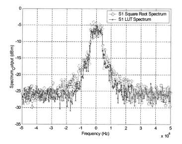
Figure 2. 20 S<sub>1</sub> spectrum comparison between LUT and SRFB
