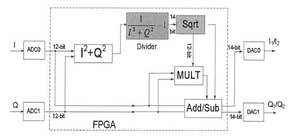
Figure 2. 11 Method 2 - Square-Root Function Block design diagram
