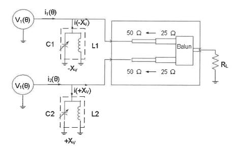
Figure 3.9 Implementation of variable reactive termination combiner
