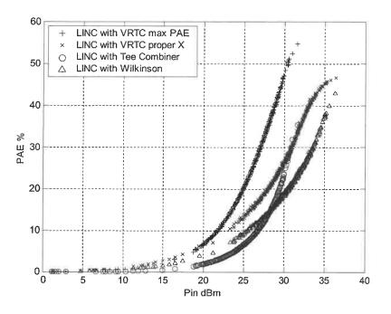
Figure 3. 13 PAE curves with IS95 signal
