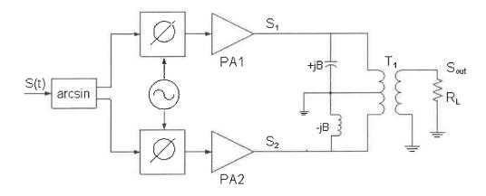
Figure 1.2 Analog LINC transmitter
