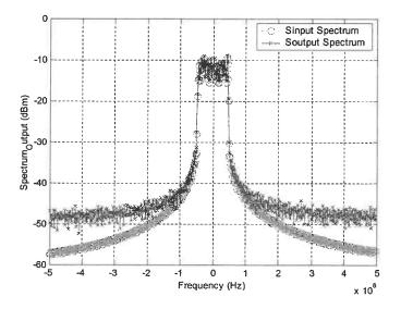
(b) LINC output  $\mathbf{S}_{output}$  and input signal  $\mathbf{S}_{input}$
