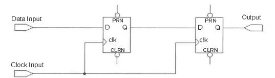
Figure 2. 6 Multiple-stage synchronizer
