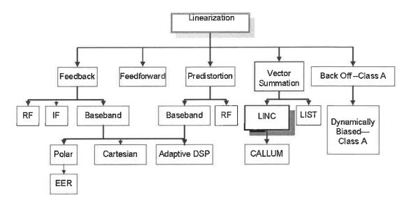
Figure 1.1 RF amplifier linearization techniques
