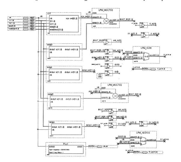
Figure 2.10 Top level design for I<sub>1</sub> (n) & Q<sub>1</sub>(n) with LUT in Quarus II 2.0
