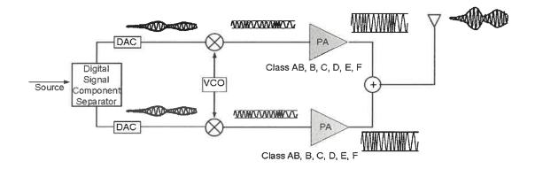
Figure 1.4 LINC transmitter using DSP technique
