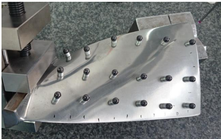
Fig. 4.26: Turbine blade with material markers [47]
