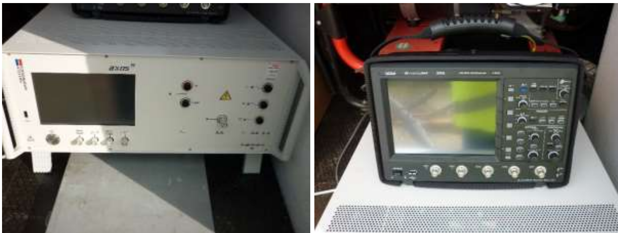
Figure 2.32 Haefely Axios 5 impulse generator and WaveJet 324A oscilloscope.
