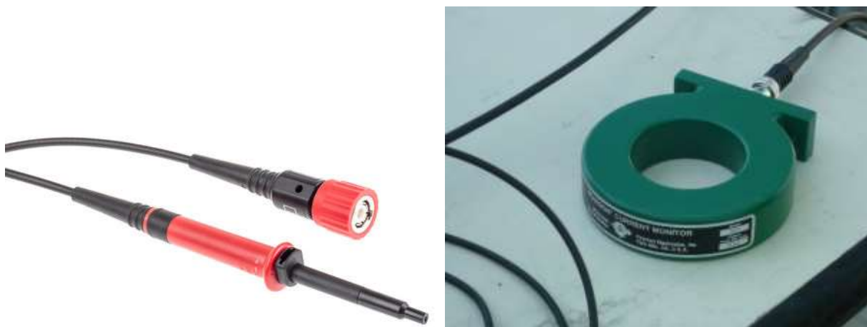
Figure 2.33 PHV1000 voltage probe and Pearson 110 current probe.
