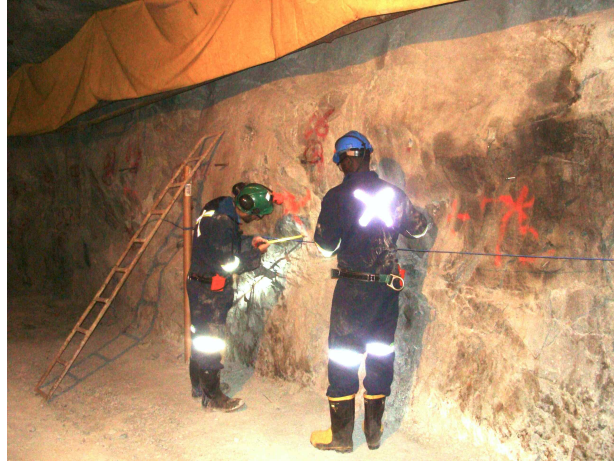
Figure 4.3 Wall surface height measurement at 40 m mine gallery.
