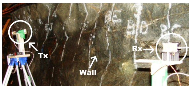
Figure 4.12 Reflection measurement campaign of the wall.
